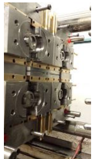
With DT Cores, no hydraulics or external core pull mechanisms are required.
