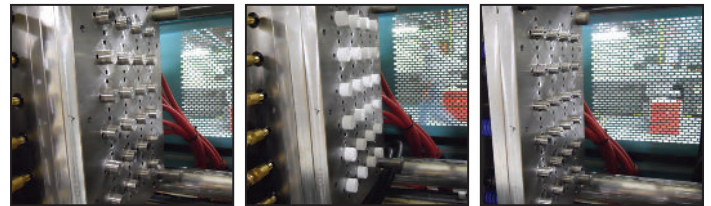
With DT Cores, no hydraulics or external core pull mechanisms are required.
